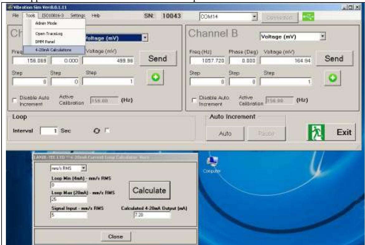
To open 4-20mA Current Loop Calculation Panel:
